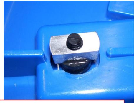
Retaining Nut Aligned for Inner Shell Removal
